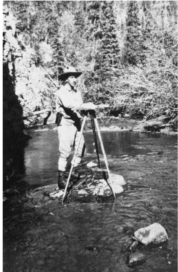
Ted Link plane table surveying up Vermillion Creek, Fort Norman area, NWT Glenbow Archives NA-5056-13
